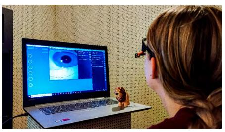
Figure 1. Example of use of eye tracking glasses for pupil size measurement.
