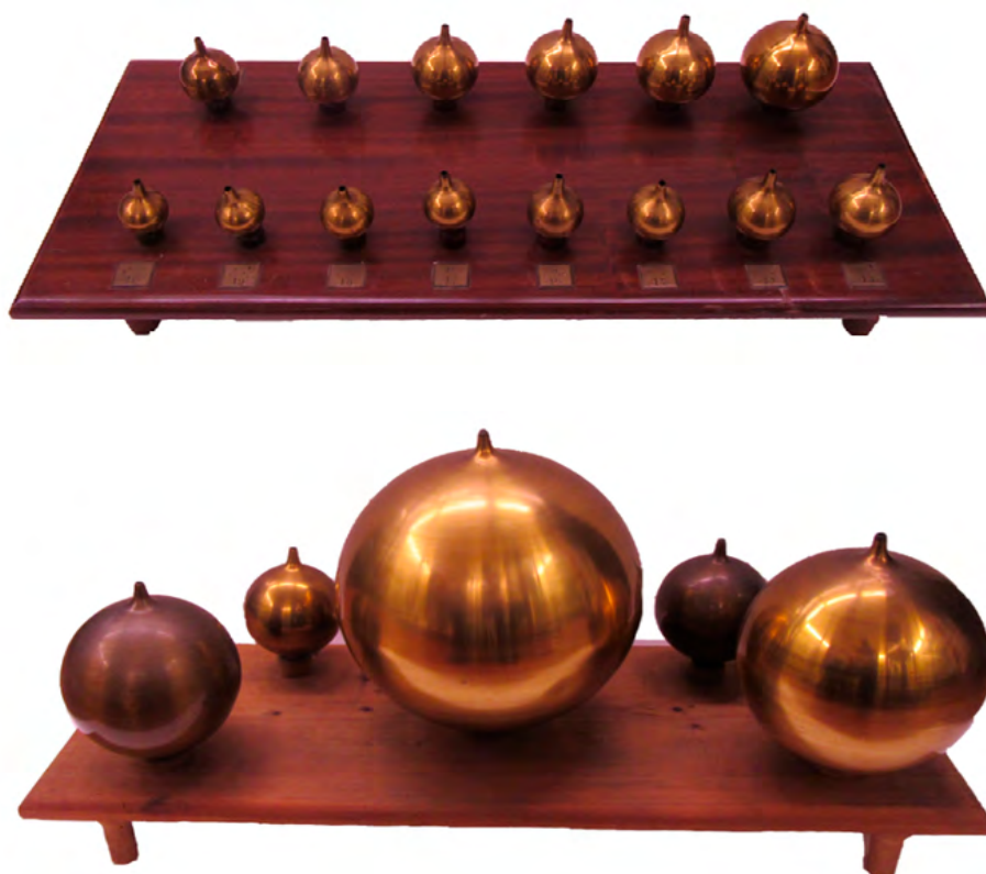
Fig.1 a,b: Helmholtz's resonators – by the courtesy of Dr. Sofia Talas, Institute of Physics, University of Padua
